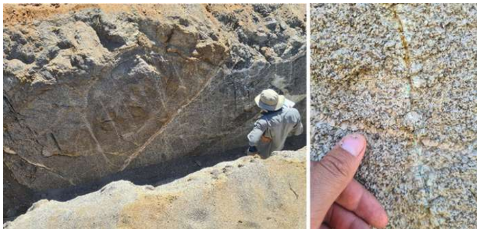
Left: View of trenching showing sheeted and stockwork fracturing. Right: Green Cu oxide and Fe oxide on individual fracture surface.
