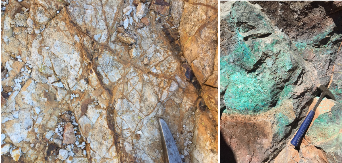
Figure 3: Porphyry style fracturing in outcrop at the base of the Especularita litho-cap alteration zone (l) and fracture-hosted secondary copper mineralisation in volcanics immediately adjacent to the contact of the litho-cap alteration.
