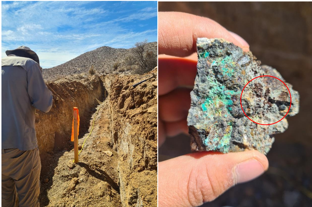
Figure 2: GSC geologist mapping trench CET009 (l). Oxide copper (green) on fractures in monzonite with evidence of goethitic box-works (after sulphide – inside red circle).
