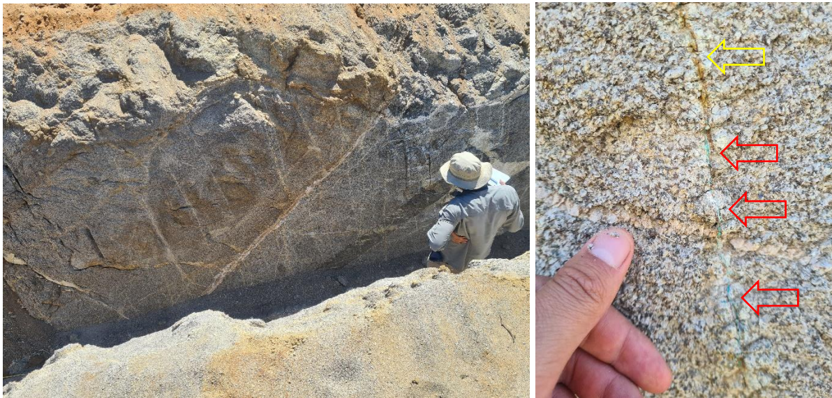
Figure 4: Sheeted and stockwork fracturing of ICP altered biotite granodiorite in trench CET002 (l). Green Cu oxide (red arrows) and Fe oxide (yellow arrow) on individual fracture surface in CET002 (r).
