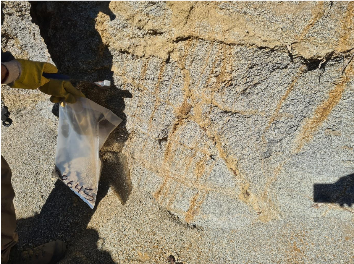
Figure 6: Sampling of highly oxidised sheeted veins from trench CWT002 location in the Chinchillon project zone. Sample 508645 recorded weakly anomalous copper in assays of 310ppm Cu, 0.038ppm Au and 0.13ppm Ag despite the intense oxidation.
